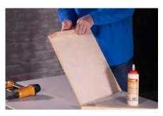
**2.** Next, glue and nail the two wedge pieces to the underside along each side.
