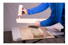
10. Then, glue and nail the cleats from the topside along the length of the board. (Tip: It may be easier to slide one side of the workpiece off the edge of your worktable to nail the ends of the 1 in. x 3 in. piece, then spin it around and do the same for the other side. Then, you can simply flip it over to nail the boards from the top.)
