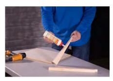
**3.** Follow this by fixing the 1 in. x 1 in. support in place between the triangle-shaped wedges along the tail end.
