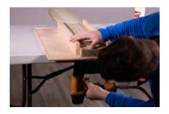
11. Flip the board over again and place the first workpiece on the second, and line them up 1 ½ in. off of the front and left side of the larger, second piece.
