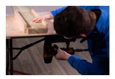
9. Next, align the 1 in. x 3 in. cleats up along the outside of the outer lines.(The measurement between the 1 in. x 3 in. boards should be 5 ½ in.)
