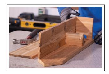
**9.** Glue and nail the front board to the assembly.
