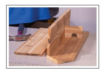
**8.** Glue and nail the bottom board to the assembled back and side, <sup>5</sup>/<sub>8</sub> in. from the bottom.
